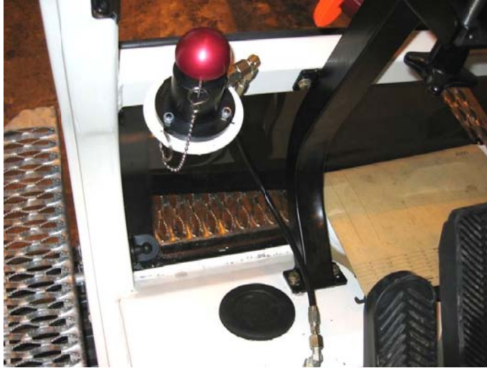
Striker button release in the driver's cabin.
