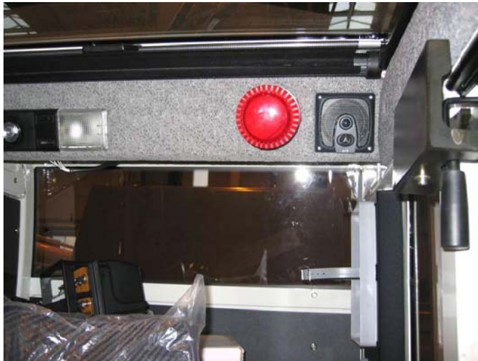
Acoustic / optical warning device in the driver's cabin.
